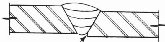
(c) Incomplete Penetration due to Internal Misalignment
